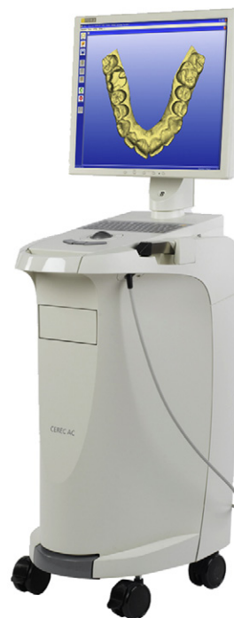
FIGURE 11.6 Chair-side CAD/CAM system for all-ceramic restorations fabrication. (Courtesy of Sirona Dental Systems, LLC, Charlotte, NC)
