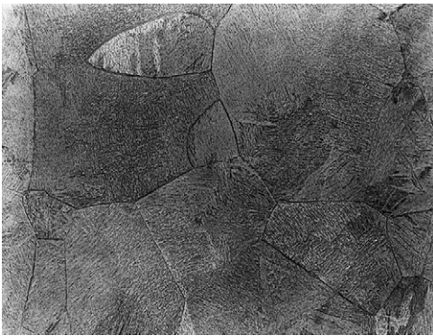
FIGURE 10.14 Microstructure of as-cast Ti-6Al-4V.
