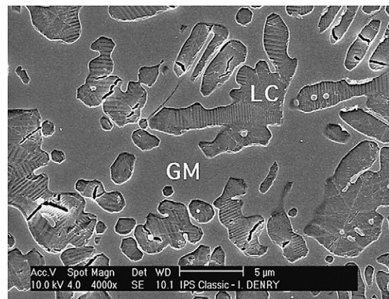
FIGURE 11.13 Scanning electron micrograph showing the microstructure of feldspathic porcelain for metal-ceramic restorations. GM, Glassy matrix; LC, leucite crystal.
