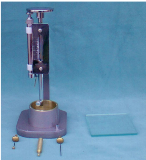
FIGURE 12.16 Vicat penetrometer used to determine setting time of impression materials and other restorative materials.
