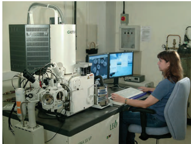
Figure 9-50 The scanning electron microscope. In an SEM, the specimen is scanned by a beam of electrons brought to a focus on the specimen by the electromagnetic coils that act as lenses. The detector measures the quantity of electrons scattered or emitted as the beam bombards each successive point on the surface of the specimen and controls the intensity of successive points in an image built up on a screen. The SEM creates striking images of three-dimensional objects with great depth of focus and a resolution between 3 nm and 20 nm depending on the instrument. (Photograph courtesy of Andrew Davies.)
